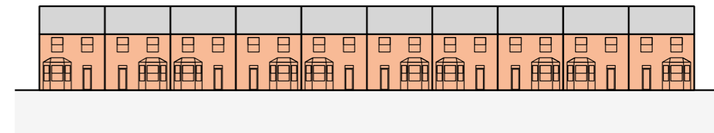
Fig. 163: Individual planning applications which increase the height of houses within a terrace of consistent character will not generally be supported.
