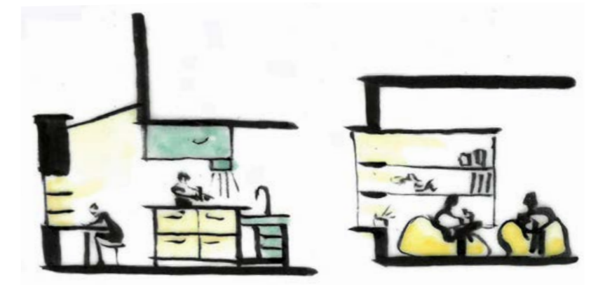
Fig. 50: High ceiling and large fanlight, good daylight to worktop and desks, well-lit living areas
